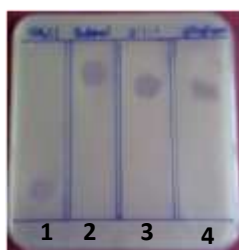
Figure 1 Paper chromatography bioautographic assay
